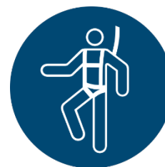
Personal fall protection when edge protection is not feasible
